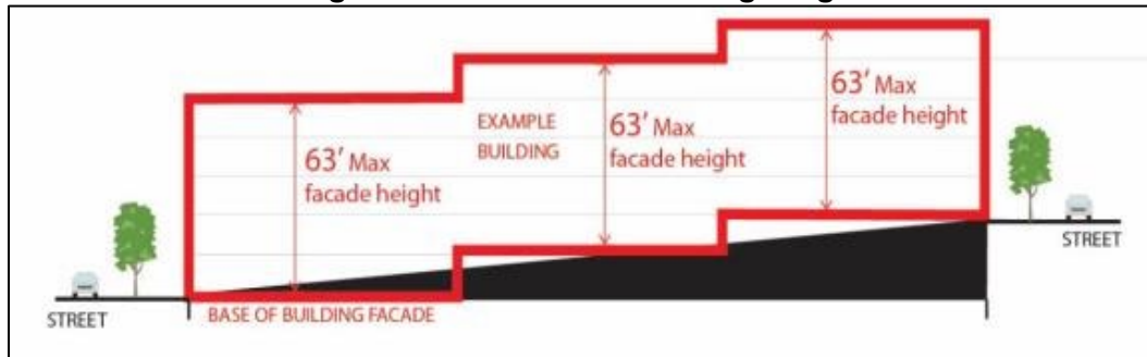
Figure 4 — Maximum Building Height
